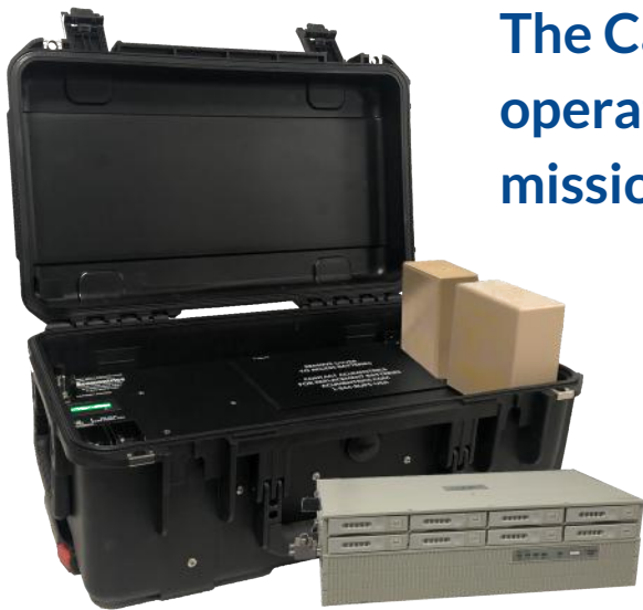
Example shown above: Mercury's RESmini XR6, a Data Center in a Briefcase
